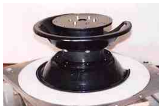
Photo 1 Isolator with buckling protecting plate
