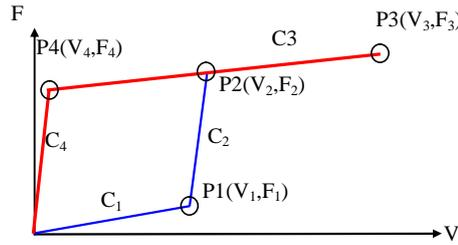
**Figure 8. Control points of variable damper**
