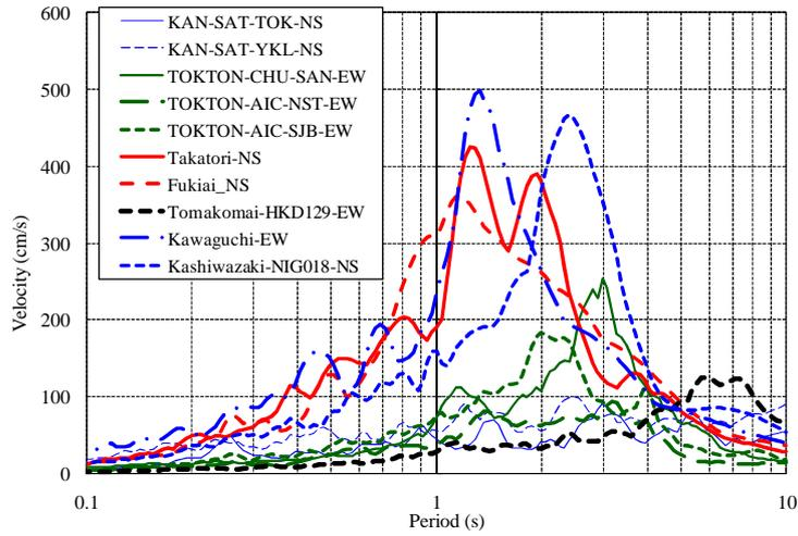
Figure 1. Pseudo velocity response spectra (damping factor = 5%)
