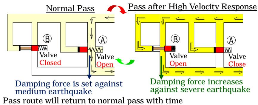
Figure 5. Characteristics of oil flow of variable damper
