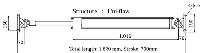
Figure 6. Schematic view of variable damper
