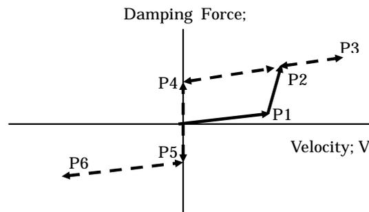
Figure 4. Force vs. velocity characteristics of variable damper
