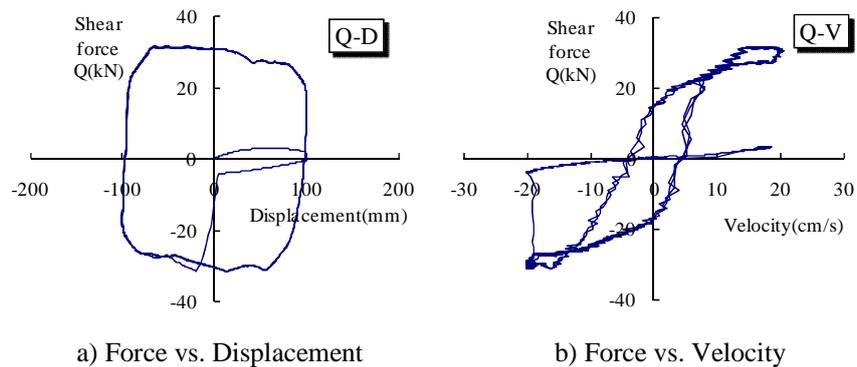
**Figure 7. Force vs. displacement characteristics under dynamic oscillation**
