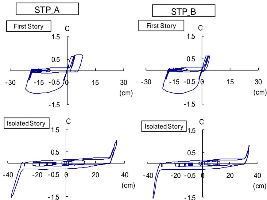
**Figure 3. Example of response of S-hv50 ( superstructure: slip, EQ : Kawaguchi-EW )**
