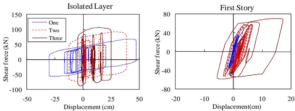
**Figure 9. Shear force vs. displacement at isolated layer and 1<sup>st</sup> story (system; S-hv0, superstructure; trilinear, EQ : Tkatori-NS)**
