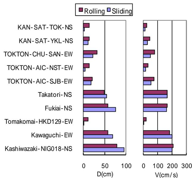
**Figure 2. Maximum relative displacement and velocity response of isolated layer**
