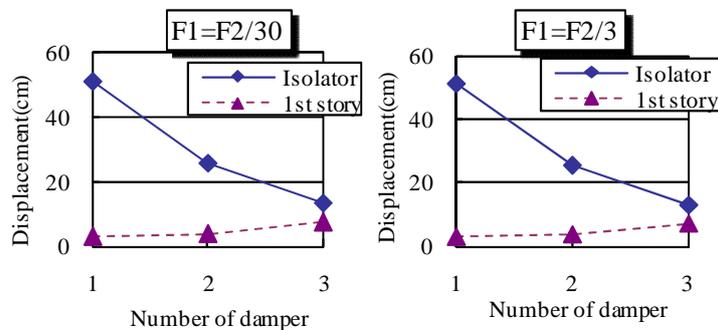
**Figure 10. Maximum Displacement at isolated layer and 1<sup>st</sup> story (system; S-hv0, superstructure; trilinear, EQ : Kashiwazaki-NIG018-NS)**
